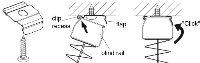
Insert the edge of the blind rail diagonally into the clip recess, then straighten upwards until the rail 'clicks' into place.
