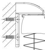
**Dismantling:** Remove the blind rail from the Fixing Clips by pushing the flaps upwards, then dismantle the Face Brackets as described below.
