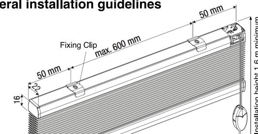
Install Fixing Clips 50 mm from each end of the rail, and with a maximum spacing of 600 mm between clips.
